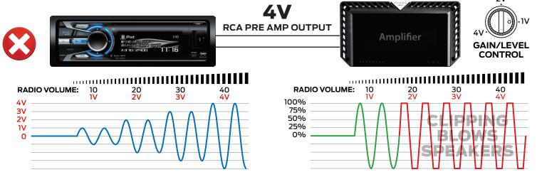
Lines in red mean too much gain, causing burnt subs/midranges/tweeters and amplifier overheating. Also cuts overall performance up to 75% when head unit volume distorts at level 25 to 40.
