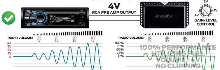
Ideal setup is to utilize full volume for full output line voltage with no clipping. See chart on reverse side for accurate crossover points.
